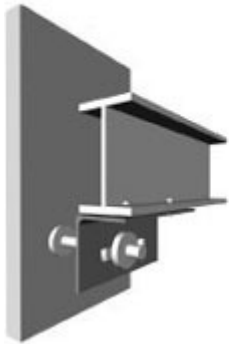
slotted hole lateral connection
