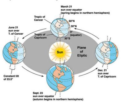
The different seasons are due to the Earth's Declination. When the northern hemisphere is tilted towards the sun, the path of solar radiation through the atmosphere is at its shortest and closest to perpendicular: Summer. When the northern hemisphere is tilted away from the sun, the path of radiation through the atmosphere is longer and at a more oblique angle to the ground.
