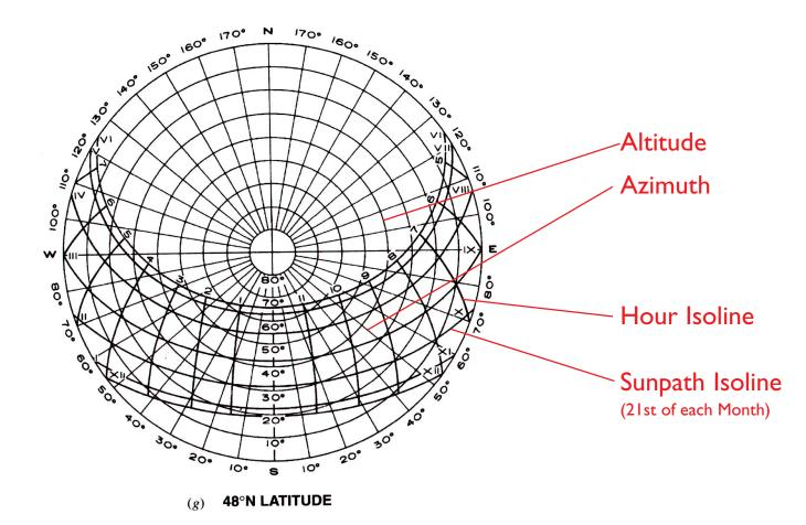
This week... <u>Thermal Control | Solar Geometry and Shading Devices</u>
