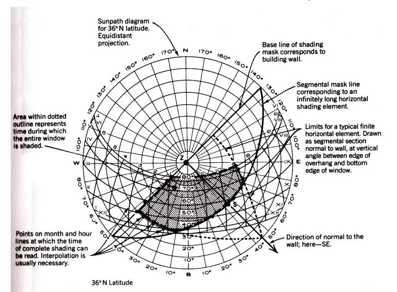
This week... <u>Thermal Control | Solar Geometry and Shading Devices</u>
