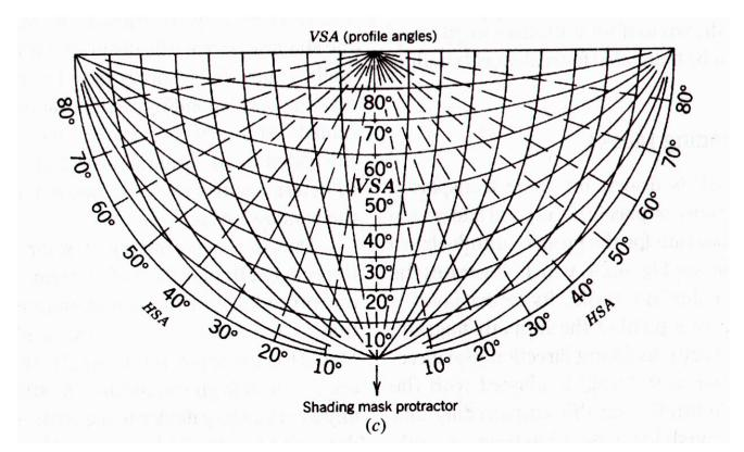
This week... <u>Thermal Control | Solar Geometry and Shading Devices</u>
